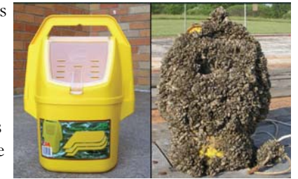
Before and after picture of object submerged in water body with Zebra Mussels.
